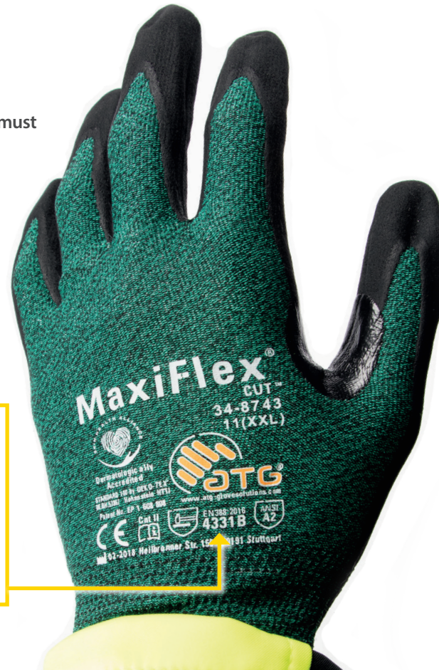
The glove to the right is classified in accordance with EN388 with protection level 4331B (it is not labelled with the last letter, and has therefore not been tested for impact protection).
